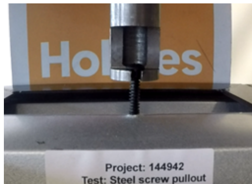
Figure 5-2. Carlisle HP-X fastener pulling out of ST900 sheeting
