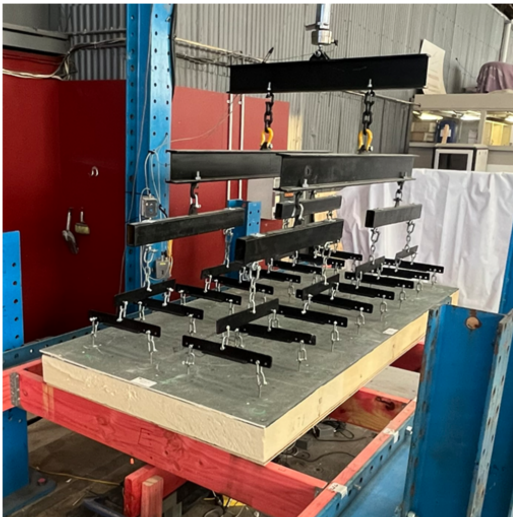
Figure 9-1. Whiffle tree attached to specimen
