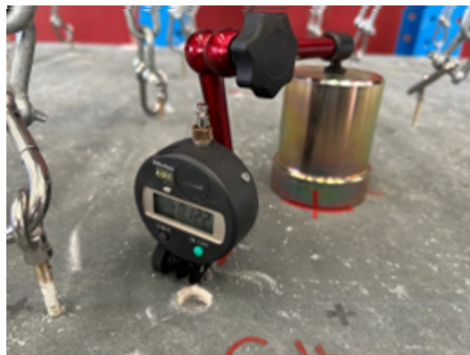
Figure 9-14. DTI measuring washer head movement during a test
