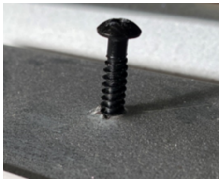
Figure 5-3. Carlisle HP-X fastener showing upturned lip
