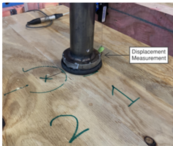
Figure 8-6. Example of point load application and measurement
