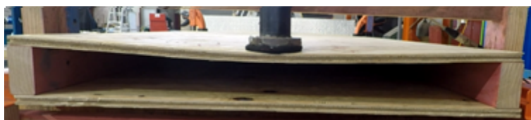
Figure 8-7. SLS deflection (Location 3, Sample 3)
