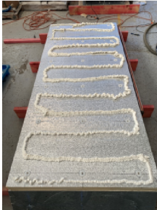
Figure 9-9. Viking Soudafoam applied to PIR panel
