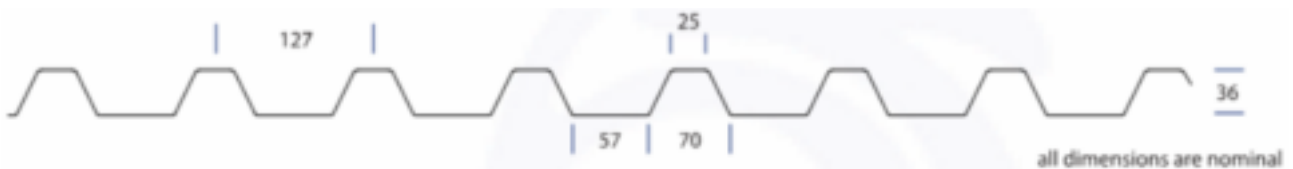
Figure 3-4. Alternative acceptable profile - Metalcraft Metcom 7 profile (shown opposite to installed orientation)
