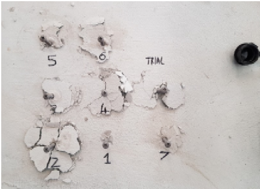
Figure 5-6. Carlisle HD14-10 fasteners after loading in concrete
