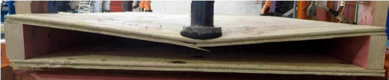
Figure 8-11. Rupture under ULS load (Location 3, Sample 3)
