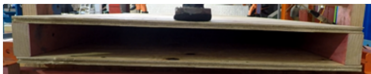
Figure 8-8. SLS residual deflection (Location 3, Sample 3)
