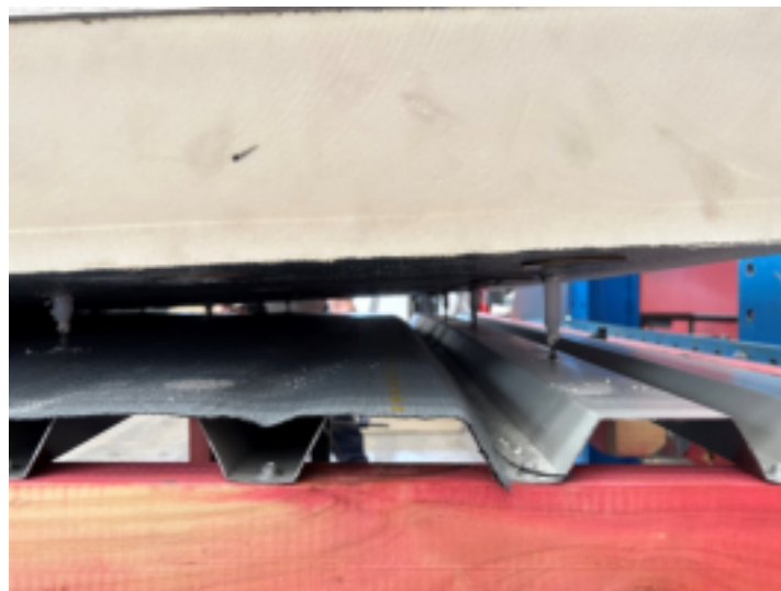
Figure 9-20. Washer pulling through PIR (during post-test removal)
